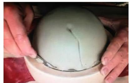
Make sure the join remains horizontal. Leave the ball inside the mould.
